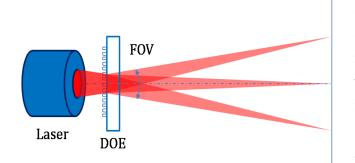
A DOE functions with a laser light source that emits a diffractive pattern. Each DOE pattern is characterized by a specific laser wavelength, focal length and transverse mode. Each laser wavelength will result in a different zero order intensity. The focal length is dependent on the DOE and the object distance which can be adjusted using a collimating lens (CL). The transverse mode will affect the dot shape.
